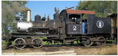
1912 HEISLER 36-TON GEAR-DRIVEN STEAM LOCOMOTIVE
