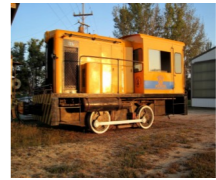
Built in 1938 by the Plymouth Locomotive Works in Plymouth, Ohio. Powered by a Buda gasoline engine. Donated by Rockford Blacktop in Rockford Illinois.
